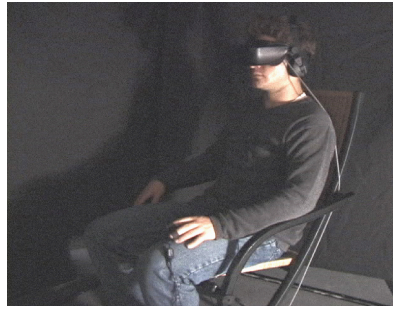
Figure 3.1 Users wear a head-mounted display, providing them stereoscopic imagery and sound. Interaction primarily occurs by users as they strive to manipulate their physiological states via biofeedback. Biometric sensors are attached to two fingers with Velcro, tracking GSR and heart rate. A flexible chest band tracks respiration.
